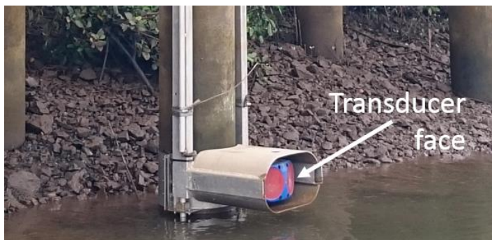
Figure 22: Example of a horizontal Acoustic Doppler Current Profiler
