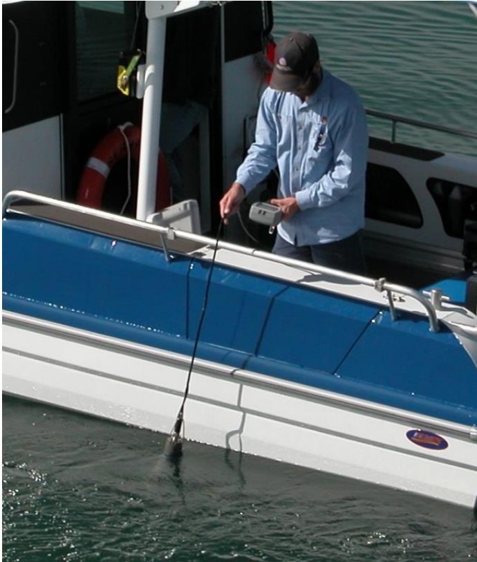
Figure 7: Testing waters with a multi-parameter water quality meter
