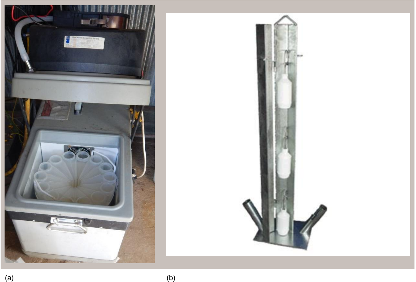
Figure 13: Automated sampling equipment: (a) refrigerated automatic pump sampler (Photo credit: DES) (b) rising stage sampler (Photo credit: Hyquest Solutions)
