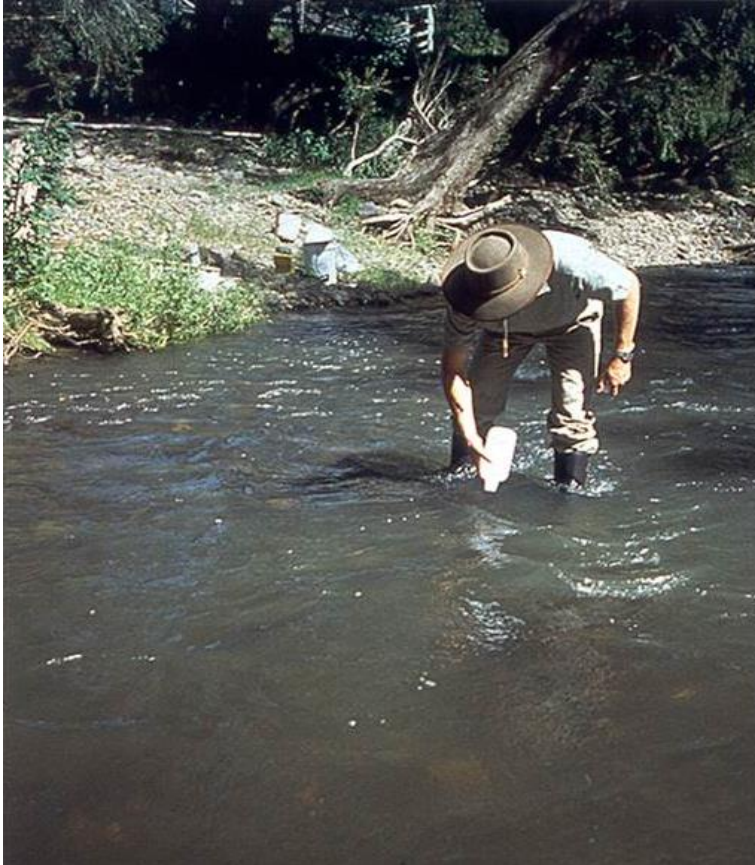
Figure 88: Collecting a grab sample
