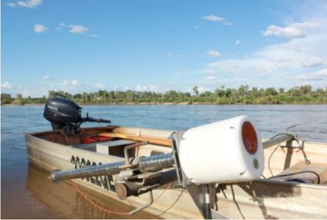
Figure 25: A boat-mounted ADCP prepared to collect velocity data
