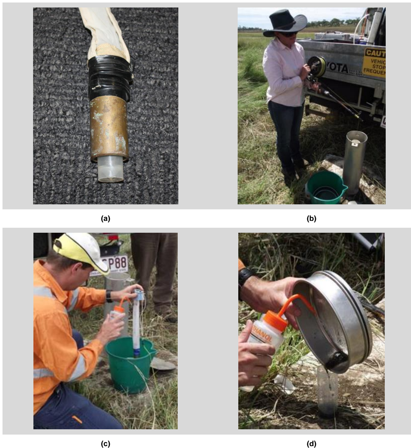
Figure 46: Sampling stygofauna using a net and reel
