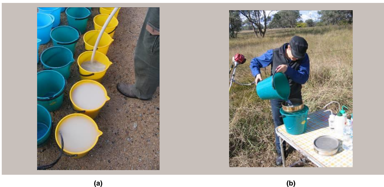
Figure 47: Sampling stygofauna using a pump and buckets
