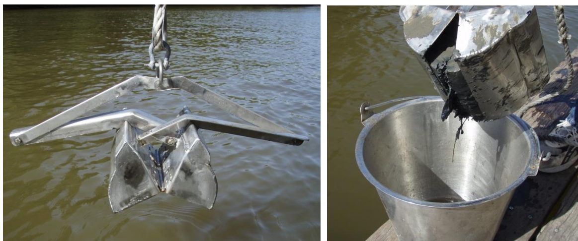
Figure 92: Van Veen Grab Sampler collecting benthic mud in sample container
