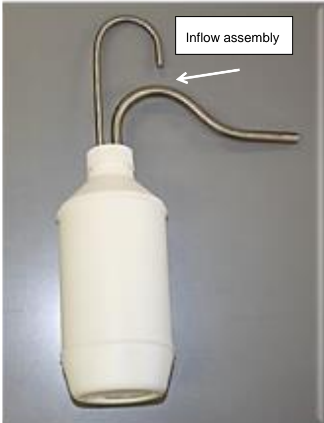
Figure 17: Stage sampler bottle with inflow assembly
