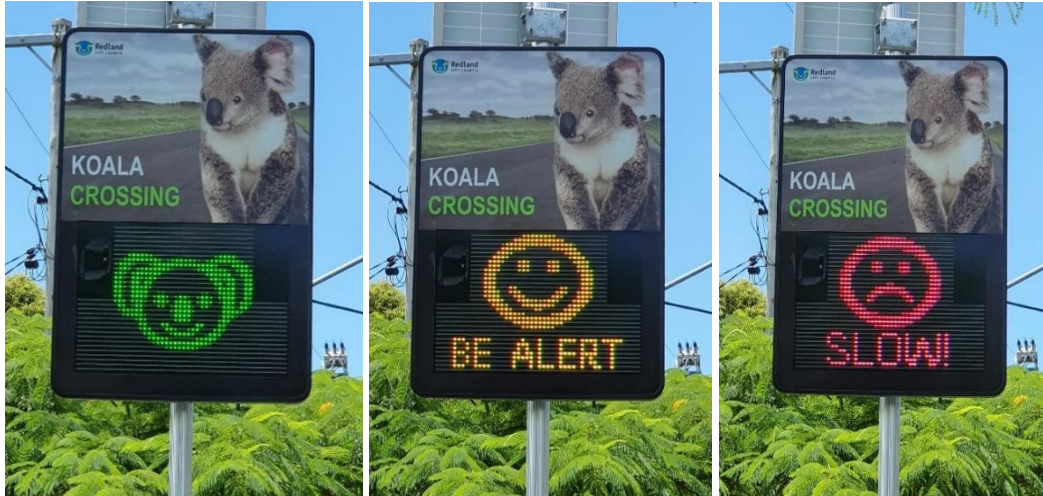
Figure 4.3.6. (photo D de Villiers) Vehicle activated signs displaying variable messaging depending on passing vehicle speed, with positive green koala smiley face when travelling below the speed limit (left), a cautionary message at the speed limit warning the driver to be alert to koalas crossing the road (middle), and a red unhappy face if the vehicle is travelling faster than the recommended speed in the conservation zone (right).
